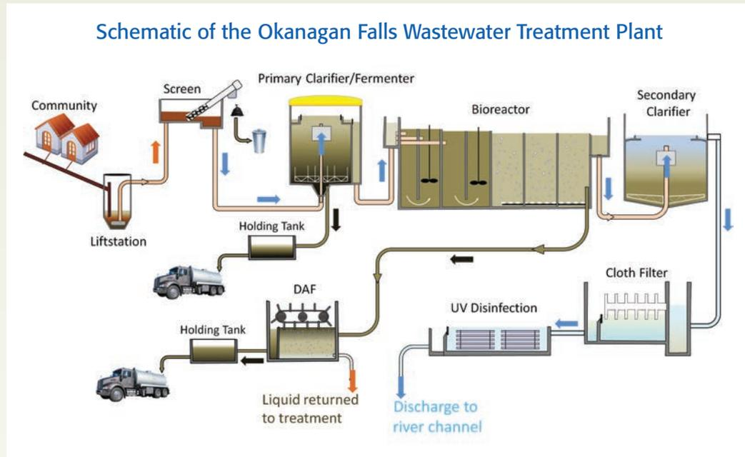
types of thickened sludge, Thickened Waste Activated Sludge (TWAS) and Fermented Primary Sludge (FPS) from the process. Currently both types of sludge are not dewatered onsite but instead hauled to Penticton's Advanced Wastewater Treatment Plant for further processing.
