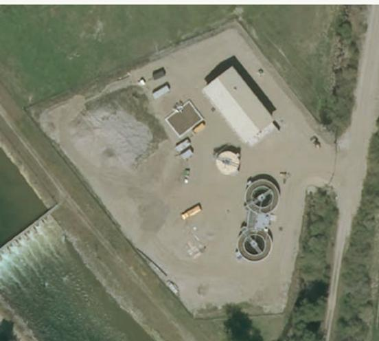
*The Secondary Clarifiers within the circular Bioreactors not only saved concrete costs, but also help conserve heat, with the Combined Treatment Units having to be 70% above ground. In addition, it is much easier for the operators to compare foaming, supernatant and visual flows within the Clarifiers and Bioreactors with them in combined treatment units.*
